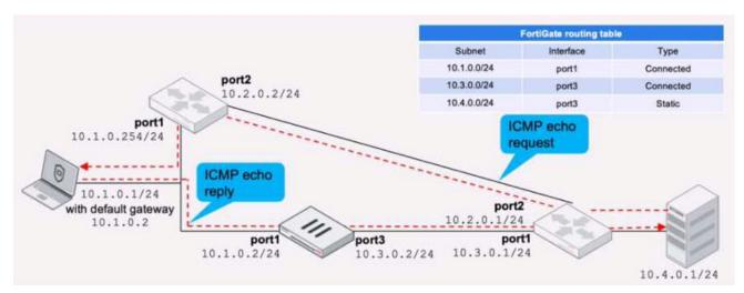
FortiGate has already been configured with a firewall policy that allows all ICMP traffic to flow from port1 to port3.
