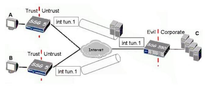
In the exhibit, the hub and spoke VPN uses route-based VPNs and has intra-zone blocking enabled on the Evil zone.
