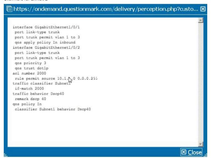
The frame shown in Exhibit 1 arrives on an HP 5800 switch's Gigabit Ethernet port 1/0/1. QoS maps are at their default settings.
