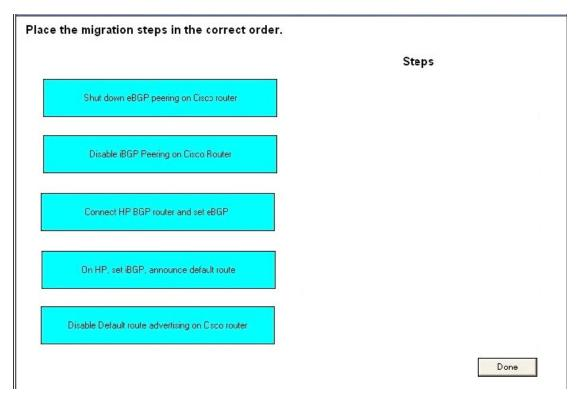
2. You want to add HP edge switches to a company's Cisco network. Distribution Cisco switches are set as
