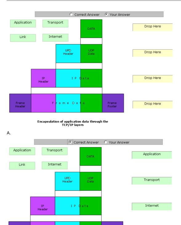
Encapsulation of application data through the TCP/IP layers
