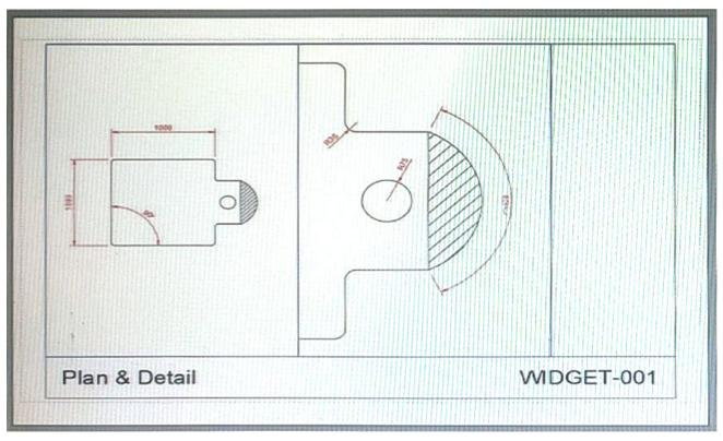
The geometry and dimensions were created in model space.
