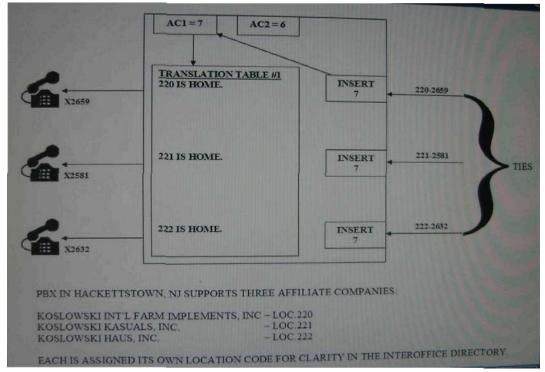
Consider a company''s dialing p an shownint he exhibit and an example for its requirements A station user at the company, with Location Code 221, placed an ESN call, dialing 7-221-2581. This would be an On-Net call and the NARS programming must remove the LOC code and dial the DN internally.
