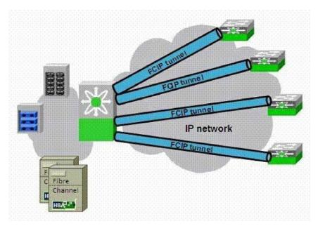
A customer is using an 18/4-Port Multiservice Module in his data center to provide FCIP connectivity to 20 remote sites. The 18/4 MSM has encountered connectivity problems at four of the remote sites. After investigating, the customer's network administrator found that the 18/4 MSM is sending 2300-byte packets, but the receiving switches at the four remote sites do not support jumbo frames. What should you do?
