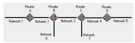
Router B uses RIP and has poison reverse enabled. Which cost metric does Router B advertise on Network 2 regarding Network 7?
