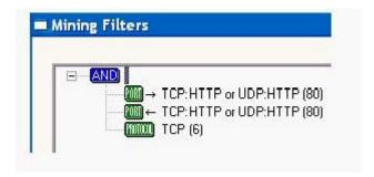
A. The filter only allows packets that are sent to HTTP servers on their well-known port. It would only show commands without replies. This filter is incomplete.
